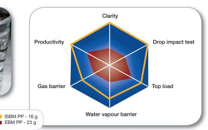
The graph illustrates the advantages of bi-orientation in the case of hollow container production: an Extrusion Blow Moulded bottle is compared to an Injection Stretch Blow Moulded one.
